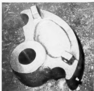
Machine bearing surfaces right in the castings... eliminate bushings, without sacrificing service.
